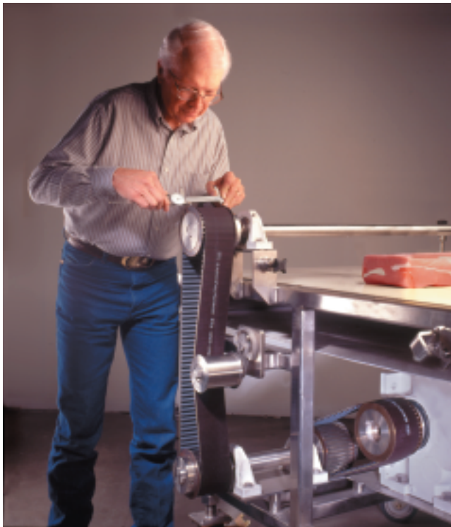
Gates engineers recommend Poly Chain® GT®2 drive systems with stainless steel sprockets because they are clean running and they resist caustic wash-down solutions.
