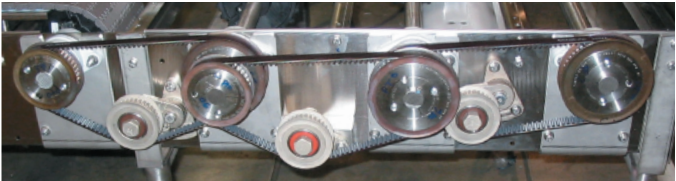
Some drive mounts may require extra plating or reinforcement to extend the service life of the synchronous belt system.
