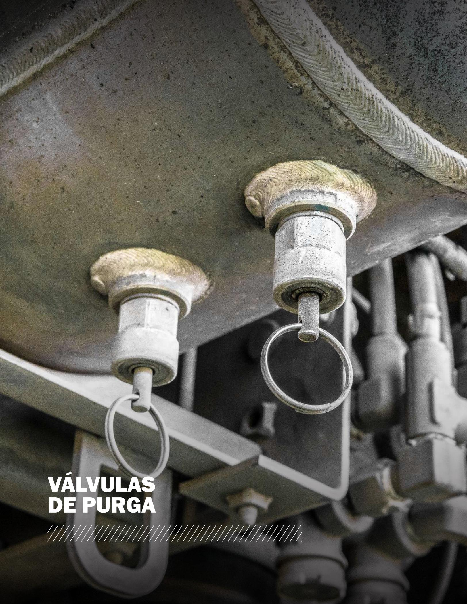
A close-up photograph of two purge valves mounted on a dark, textured metal surface. Each valve has a brass-colored, knurled top cap and a silver-colored cylindrical body. A metal ring handle is attached to the bottom of each valve. The background shows various mechanical components and pipes, suggesting an industrial or automotive setting.
